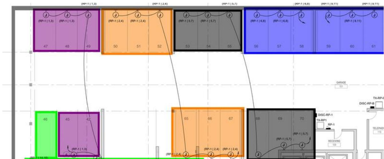
Fig. 2 Example of actual layout of several groups of EVSE chargers in garage.
